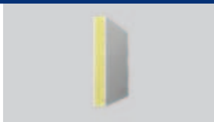
Thin partitions designed as uprights with steel substructure and clad on both sides with non-combustible structural panels
