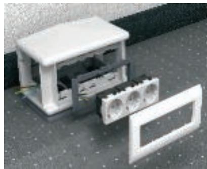
Installation of Modul 45 devices in T4L and T8NL Prepare the cable openings in the Telitank T4L mounting box and lock it into the housing. Before connecting cables, lock the Modul 45 device in the cover plate.
