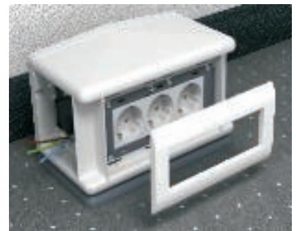
Installation of Modul 45 devices with S990 covers in T4L and T8NL Prepare the cable openings in the Telitank T4L mounting box and lock it into the housing. Before connecting cables, lock the Modul 45 device in the Telitank adapter. Lock the S990 cover plate in the housing from the outside.
