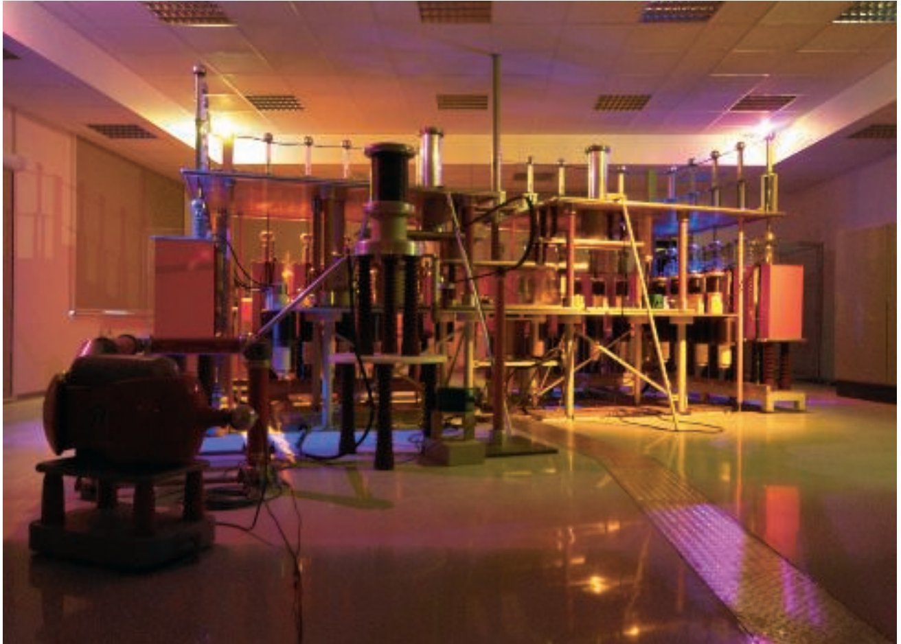
Lightning current test
