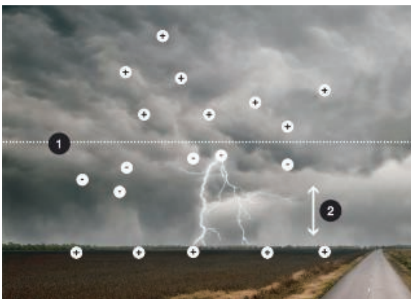
Charge distribution: 1 = approx. 6,000 m, 2 = Electrical field
